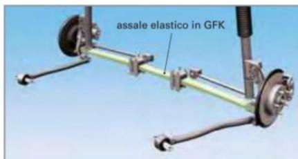
Figura 2: Assale posteriore in GFK
