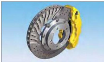
Figura 3: Disco freno in CFK
